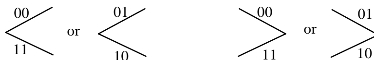
Figure 47. Diverging and Converging Branches for Trellis Branches in 64-State, Rate 1/2, Convolutional Code.
